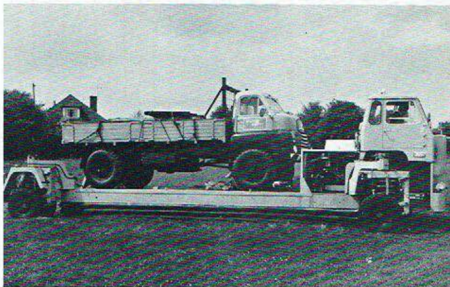
Off-the-Road Transporter carrying a 9 ton load over soft open country.
