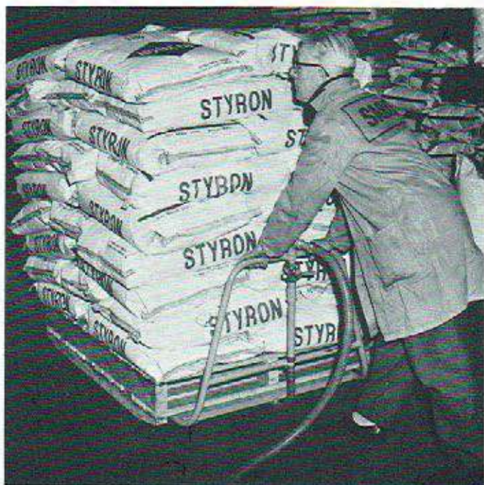
A loaded 1 ton Hoverpallet. For handling goods in many branches of Industry.
