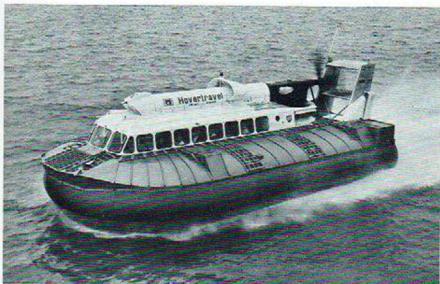
One of the 38 seat Winchester Class SR.N6's on regular service over the Solent, between Portsmouth and Ryde, Isle of Wight.
