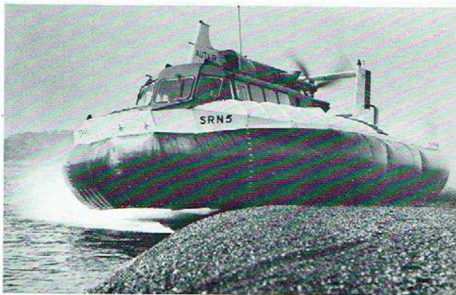
Amphibious versatility illustrated by a 7 ton 18 seat Warden Class SR.N5.
